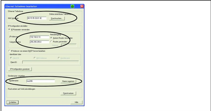
Figure 3.4: MAC address - IP address -individual device name
