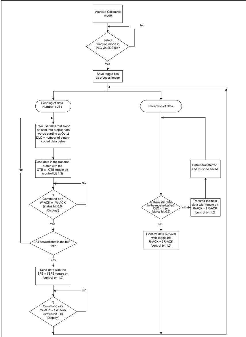
Figure 11.1: Data transmission scheme with long online commands
