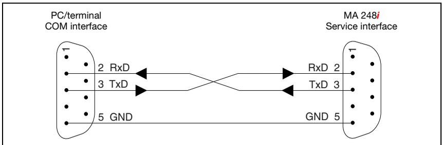
Figure 7.7: Connecting the service interface to a PC/terminal
