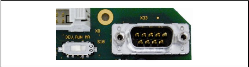
Figure 7.6: RS 232 service switch and service interface
