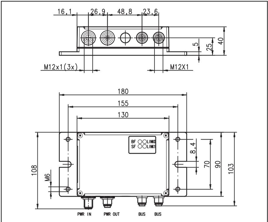
Figure 5.1: MA 248i dimensioned drawing
