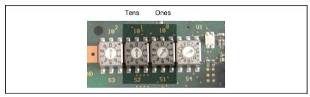
Figure 3.2: Rotary switch for setting the address
