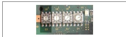
Figure 12.2: Rotary switch for setting baud rate
