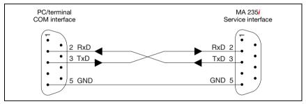
Figure 7.6: Connecting the service interface to a PC/terminal
