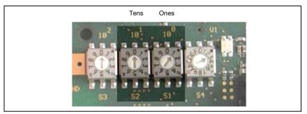
Figure 8.6: Rotary switch for setting the address
