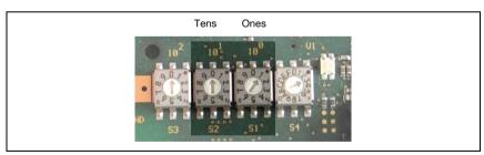
Figure 12.1: Rotary switch for setting the address
