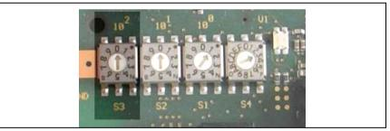
Figure 8.7: Rotary switch for setting baud rate
