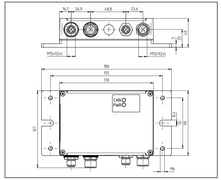
Figure 5.1: MA 235*i* dimensioned drawing
